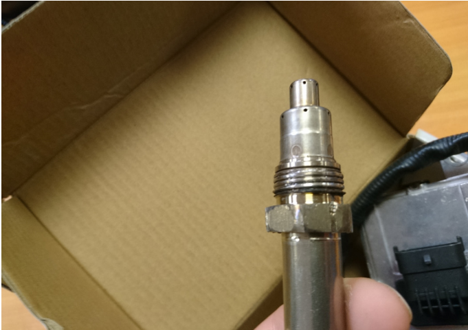
Figure 11. Damaged sensor thread and nut.
