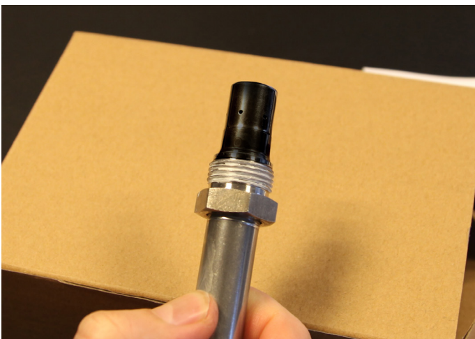
Figure 12. Evidence of excessive soot/ash.
