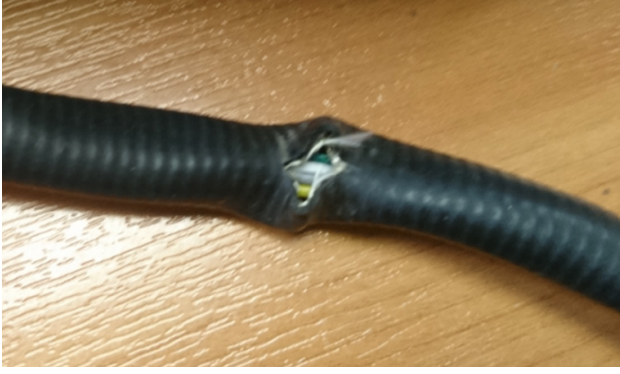
Figure 13. Damaged wire protector.
